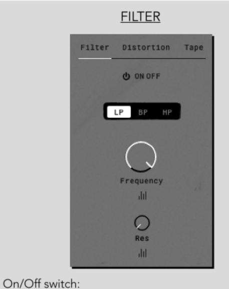
Activates/deactivates the Filter LP/BP/HP: Choose between Lowpass, Bandpass & Highness Filter Frequency: Adjust the Frequency Adjust the amount of Resonance Modulation Control: This is a quick way to check and control the amounts of modulation for the Filter Cutoof and Resonance
